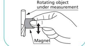
Note: Be sure to magnetize the target measurement object before starting measurement.
