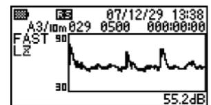
Displays level on vertical axis, time on horizontal axis.
