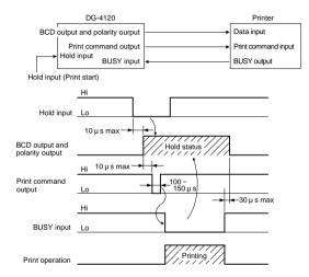
In the diagram shown above, the printer is started at the leading edge of the print command pulse signal. The hold input must be maintained at Lo level until the BUSY input turns Lo.
