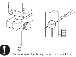
Mounting by squeezing stem using collar
