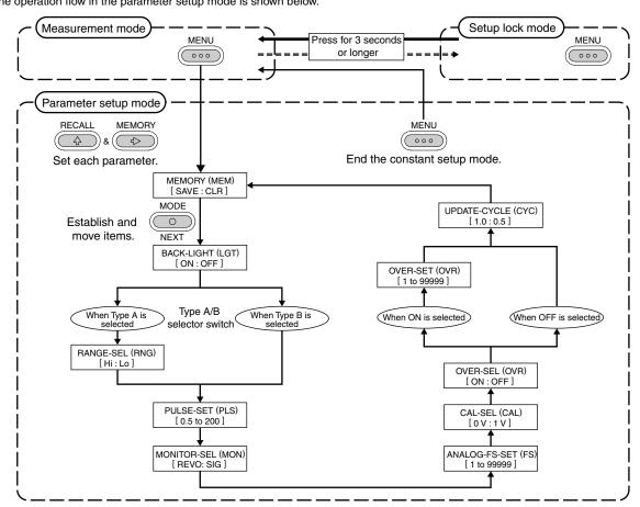
Before setting each parameter in the parameter setup mode, select the measurement mode to be used.
