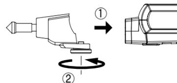
Align the contact adapter with the detecting element of the main unit and then fix it firmly to the tripod mounting screw at the bottom of the main unit using a knurling screw.
