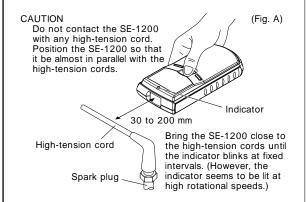
Press the power switch and then bring the detecting element close to the high-tension cords (ignition cords) of the engine as shown in Fig. A. The indicator of the SE-1200 starts blinking.
