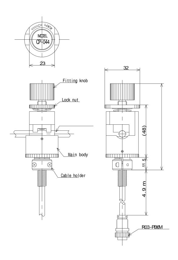
Possible external diameter of diesel fuel injection: 4 - 8
