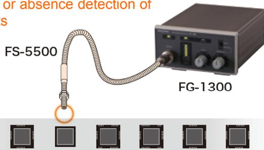
The FS-5500 can project to a small part at a pinpoint with  $\phi 2\text{mm}$  of light emission. Presence or absence of a small part flowing on a production line can easily be detected by measuring reflected light amount and judging the level of it by the threshold function.
