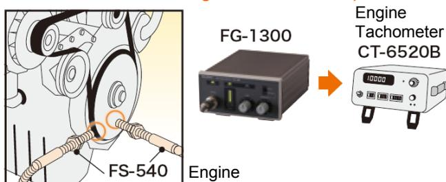
The FG-1300 performs rotational speed measurements of an engine by means of detecting reflected light from a rotating object, then outputting the light as pulses which are inputted into an engine tachometer. Marking a pulley enables measurement even if the pulley is oily which would prevent a reflective mark from sticking.
