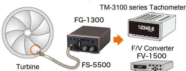
Since the FG-1300 can detect minimal change of light, it allows for rotational measurements without a reflective mark. Therefore, a turbine fan that does not directly reflect optical light can be detected. The sensor part enables the device to perform rotational measurements even in very hot temperatures where a reflective mark would not stick as in the case of a turbocharger.
