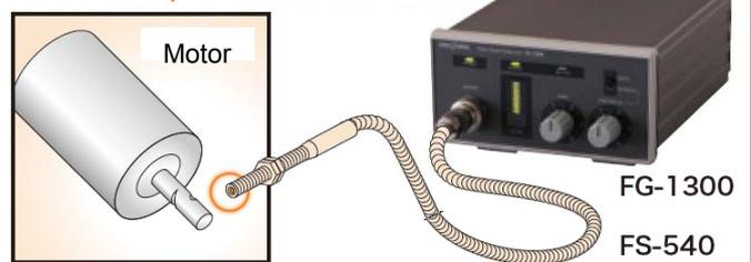
You can obtain rotational signals even from an object such as a thin shaft of a micromotor, as long as there is a 'micro-dent', uneven color or an oil-based pen marking on the surface. The FG-1300 features a maximum of 10 kHz response frequency and enables the detection of a high-speed rotation of 100,000 r/min.
