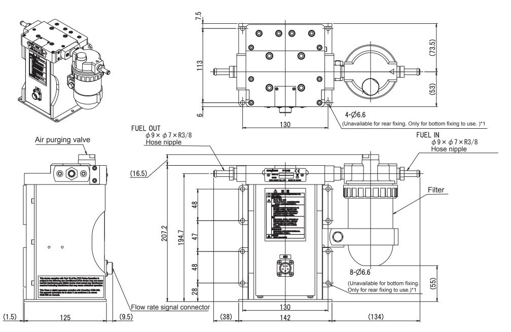
\*1: Do not fix with both sides (rear and bottom) to avoid distortion so that the measurement result will be not affected .
